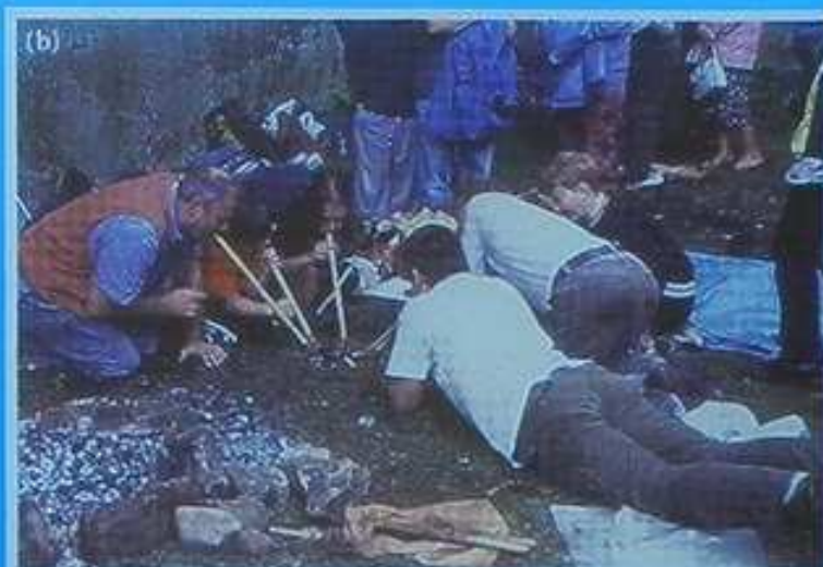
Figure 6 (a) Crushing azurite nodules and preparing the ore and fuel balls for the furnace, near Engine Vein, Alderley Edge (1997). (b) communal blowpipe smelt of a malachite/azurite ball within a small pit, Alderley Edge (1998). (Photos: P.T. Craddock.)
